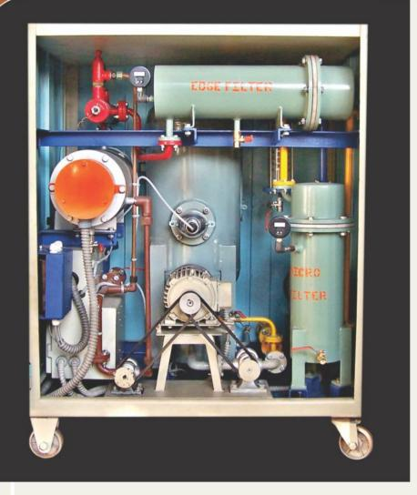
What is the essential to filter the Quenching oil? As metal is guenched in an oil shower, fines frame in the Quenching oil from the cooling procedure. Particles including carbon particles and little bits of blaze are added to the Quenching oil after some time. As these fines develop in the encompassing quench fluid, they can influence the guench in any number of wavs.
